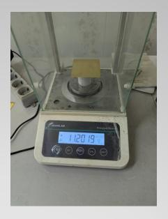
This experiment is test of nanomaterial plate. The weight is different in the case "nanosurface up" and "nanosurface down". After this test this nanomaterial must be tested in closed sealed box under high pressure gas. We use agnon. Argon is more heavy gas than air.
