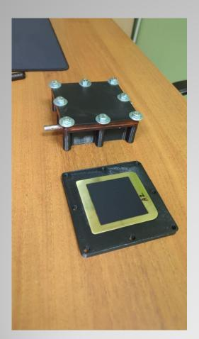
The box and the cover. Plate with nanomaterial is installed on the inner side of the cover.
