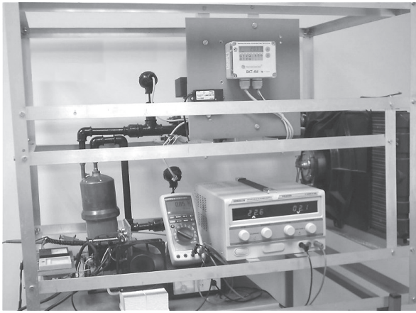
Fig. 1. The experimental device in J.L. Naudin's laboratory. A test-bench with heat calculator, a system of water cooling and ESB 3.314.363 lamp was exported from Saint Petersburg in 2004 by Faraday Lab Ltd.
